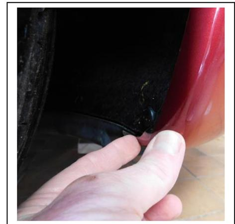
18. Apply a very small dab of RTV sealer at the very bottom end of the PPF to inconspicuously secure the PPF. This protects the PPF in this high impact area and tacks it in place.
